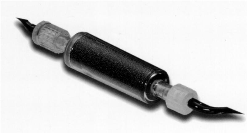
Changed weekly inline in the tubing using luer locks. A cartridge will Filter water with .22 micron membrane and maintain purity even with suckback. Emits a 2-4 ppm iodine residual at the point of use reducing cross contamination.
