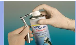
Once a week the spindle of the handpiece has to be lubricated
